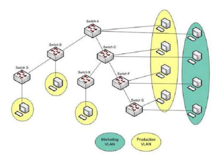
To meet a new requirement, Marketing VLAN users must communicate with Production VLAN users and vice versa. What changes would be required for the network in this scenario?
