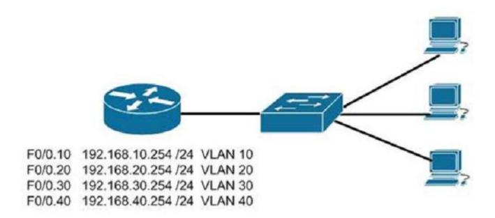
Furthermore, the physical link on the router must be subdivided into subinterfaces and addressed according to the legend shown for each subinterface in the diagram. For example, the configuration for VLAN 10 shown in the diagram would be as follows:
