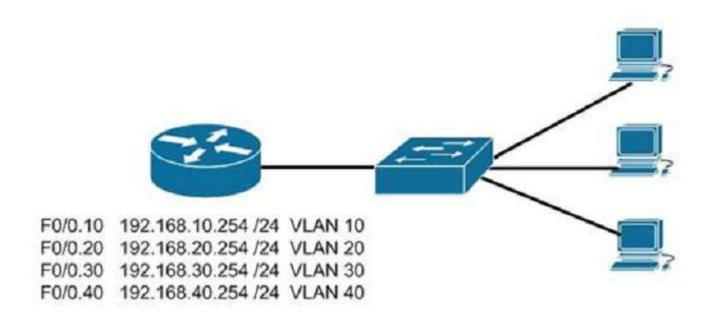
What action should you take to place the new computer in the Accounting VLAN and allow for inter-VLAN routing?
