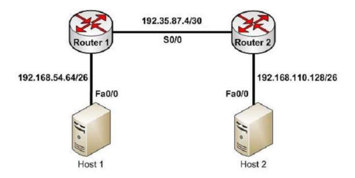
hostname router 1 hostname router 2 router rip router rip network 192.168.54.64 network 192.168.110.128 ip route 0.0.0.0 0.0.0.0 192.35.87.5 < output omitted > < output omitted >
