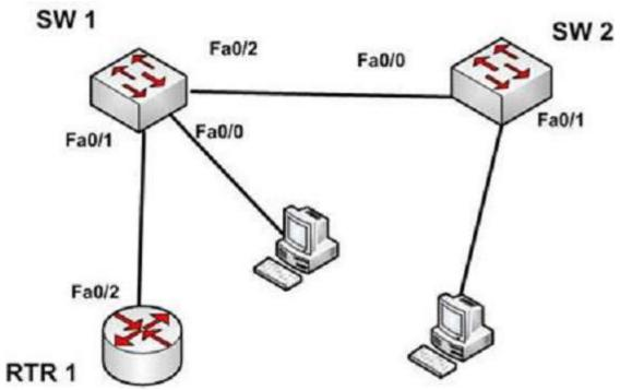
With the exception of frames traveling on the native VLAN, data frames crossing a trunk link must be frame tagged over the link to identify the VLAN that sourced the frame. The receiving switch sees the VLAN ID, and uses this information to forward the frame appropriately. 802.1q and ISL are the two possible frame tagging methods between Cisco switches. In summary, some facts about access and trunk ports:
