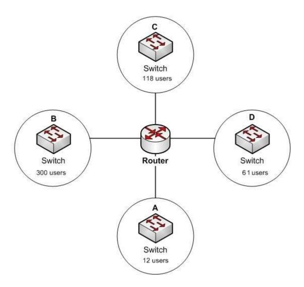
You are designing the IP addressing for this network. You are instructed not to waste IP addresses by making the subnets larger than necessary. Click and drag the correct network ID from the left to the appropriate subnet on the right.
