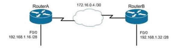
The LAN networks extending from Router A and Router B are derived from the same Class C network, 192.168.1.0/24. A classful routing protocol such as RIP v1 would not be able to determine the direction to send the packets, but since classless protocols include the subnet mask in advertisements, they would not suffer the same problem. Whenever networks with non-default subnet masks are used, a classless routing protocol will be required.
